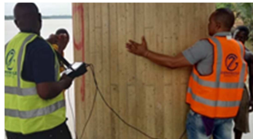
Figure 3. Testing of Piers using UPV.
